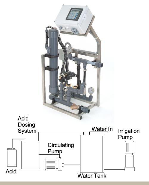
The Heron circulating acid dosing system is designed for the acidification of water storage tanks.
